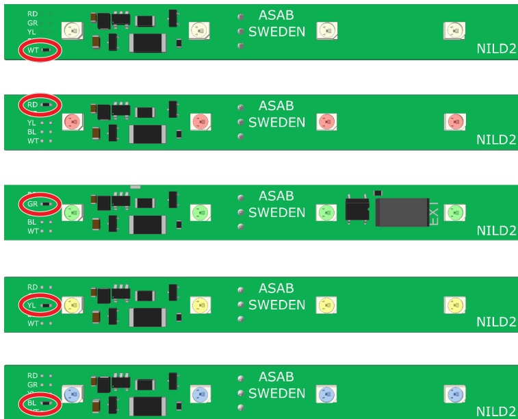
Figure 9. NILD2 - LED lamp boards: white, red, green, yellow and blue
